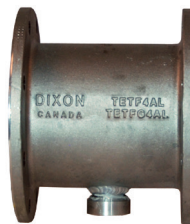
TTMA Flange, 6" Extension with 1/2" FNPT Port TETF4ALFP50
