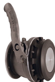
API adapter with fixed handle (poppet can open with API coupler engagement or by using the handle) 5204NG
