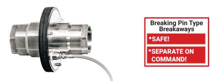
The Mann Tek Cryogenic PERC design combines the passive safety feature known from our breaking pin type breakaways with the ability to separate on command without any force on the hose. When actuated by a remote control, a pressurized gas cylinder will open and gas pressure will overcome the breaking bolts. The PERC system corresponds to standard EN1474-1:2008.
