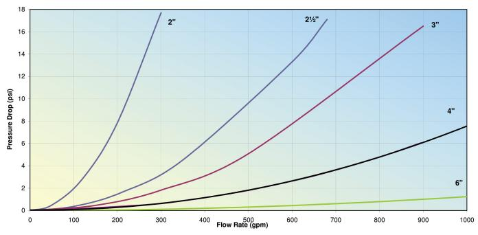
Test Fluid: LNG Temperature: -256 °F
