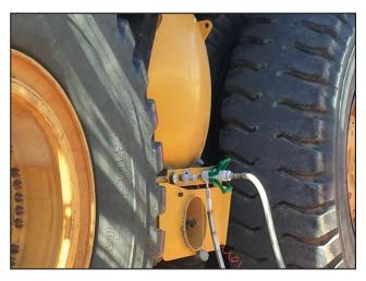
LNG fueling application on off-highway mining truck
